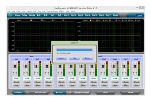
2, Connect the processor to the computer by USB, after turning on the device, the computer will searching new hardware automatically, during setup new hardware there will show the. Warnings: hardware setup success and can be used.
